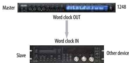
Figure 4-20: Slaving another digital audio device to your MOTU device (a 1248 in this example) via word clock. For the 1248 clock source, choose any source besides word clock, as it is not advisable to chain word clock.
