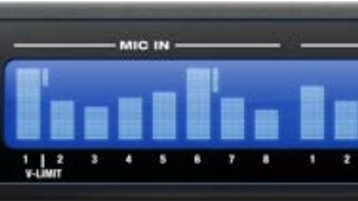
Figure 6-1: V-Limit compressor on the 8M interface.
